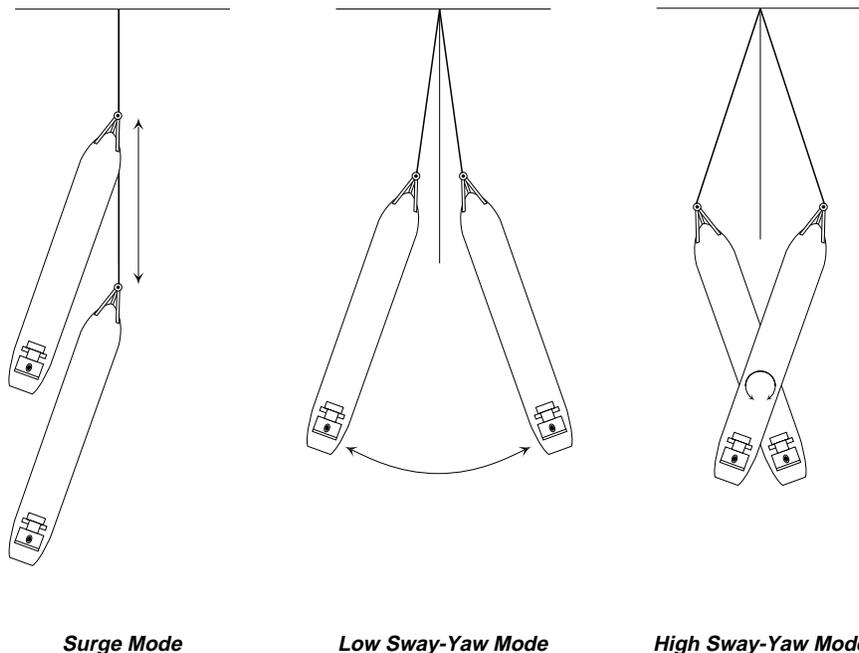
Evaluation of oscillation periods and damping of the system can be carried out once the restoring force versus offset characteristics of the mooring system are known. The system is treated as a simple quasi-linear oscillator
